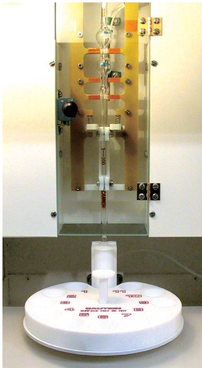
PolyVISC interior with PVDF/PTFE upgrade
